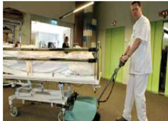
Electric support for pushing a bed.
