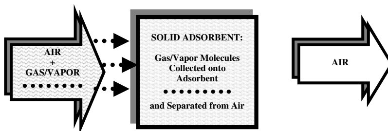
Figure 9.1 Separation of organic vapor samples from air via adsorption on a solid medium.
