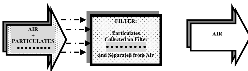
Figure 4.1 Separation of particulate sample from air via filtration.
