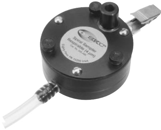
Figure 2.41 Spiral Sampler for respirable dust (a model available for PM 2.5 ). (SKC)
